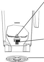
**Blade Agitator Assembly.** The blade assembly includes a precision-hardened stainless steel blade with enclosed steel ball bearings for maximum durability. The rugged blade assembly literally explodes molecules of food and ice in the container, helping every batch to homogenize more effectively. The blade does not need to be removed for normal cleaning. (Refer to the information below to remove or replace.)
